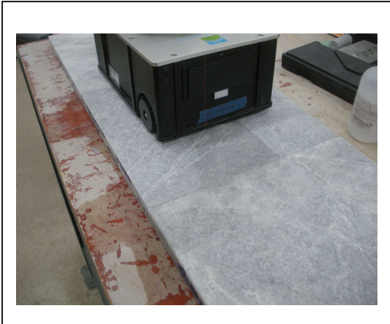
Photo No. 4 DCOF Test in Progress
