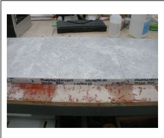
Photo No. 3 DCOF Test Set Up
