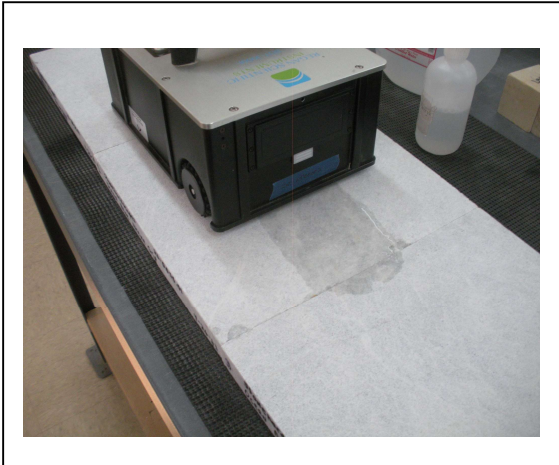
Photo No. 4 DCOF Test in Progress
