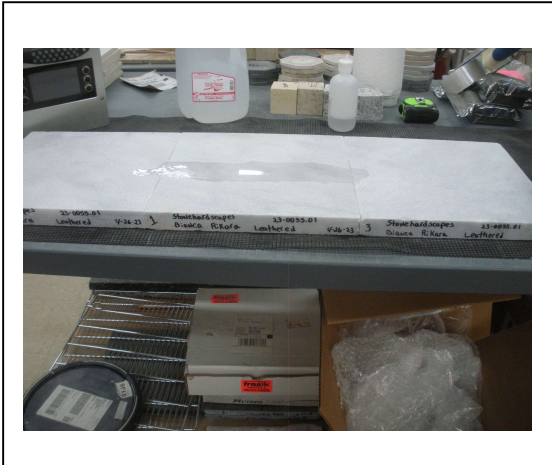
Photo No. 3 DCOF Test Set Up
