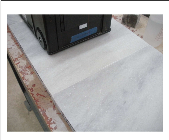
Photo No. 4 DCOF Test in Progress
